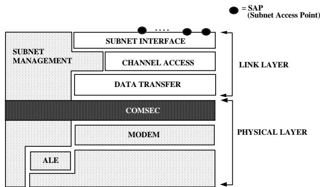
**Figure 1. Sublayers within the Profile for HF Data Communication**
