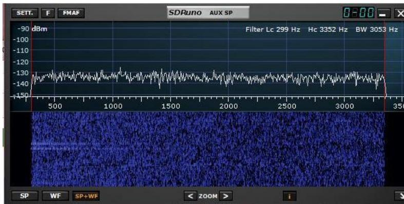
When intercepting an MS110A transmission the “SP2” window is the best to view as to the transmitting stations signal quality if in attended monitoring. We are looking to see the sending station with a bandwidth of at least 2.8kHz and no more than 3.0kHz displayed in our passband. As seen in the image below the sending station was making the grade at just about 2.8kHz on a channel with Multipath/Fading that was easily handled by MS-DMT resulting in perfect copy.
