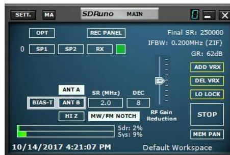
When DEC is at 1 as viewed on the “Main SP” (SP1) window when SP1 zoom is at its minimum affect the bandwidth span displayed will be at its maximum for the selected Sample Rate (SR) if the SP1 window is opened wide enough. The DEC selection of 2 will cut the SR selection bandwidth displayed on SP1 in half. Each successive DEC selection presented for the given SR selection will likewise act as a divisor in determining the provided RF bandwidth. The higher the SR the more DEC selection options.
