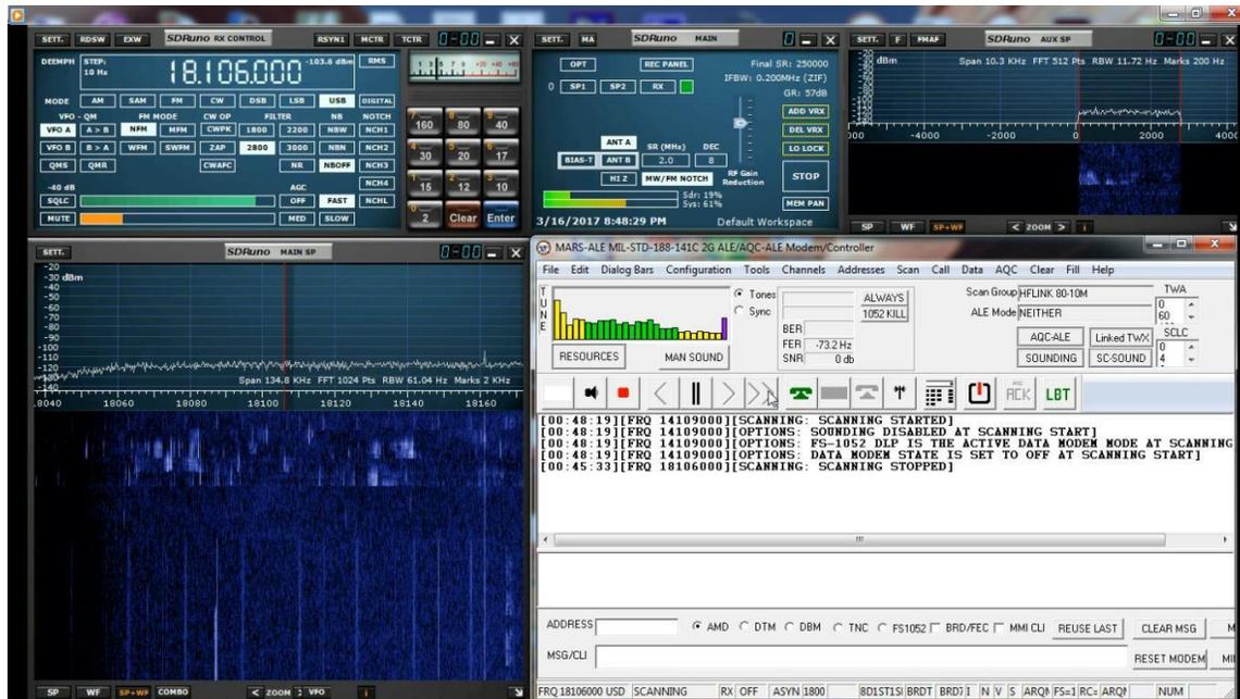
However having anything but MARS-ALE and the main SDRuno panel active after configuration is just overhead that is not required for our needs. In addition the SDRuno bandwidth should be reduced down to a minimum as the full 10Mhz results in too much CPU loading for our needs.
