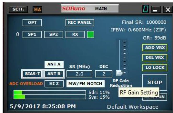
The factory gain settings are a good starting point that I have found to work well out of the box. A return to them and all factory parameters can be had with a system reset at any time, however everything is reset.
