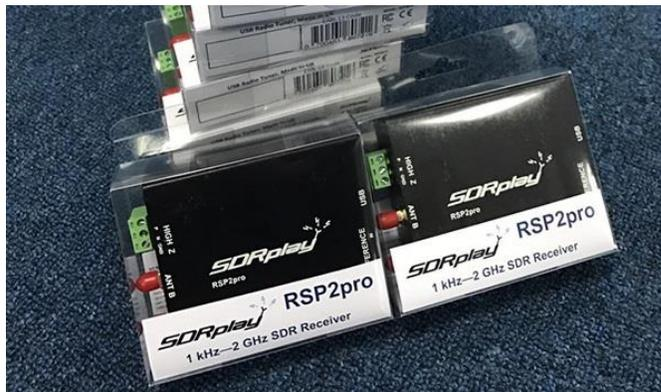
Both units real world interface consists of three selectable antenna ports on one end, where one is a Hi-Z (high impedance) for direct use with random antenna. The two 50 ohm antenna ports use standard female SMA connectors where dust covers are provided. The other end of the unit features the USB connector and MCX Clock-in and Clock-out ports.
