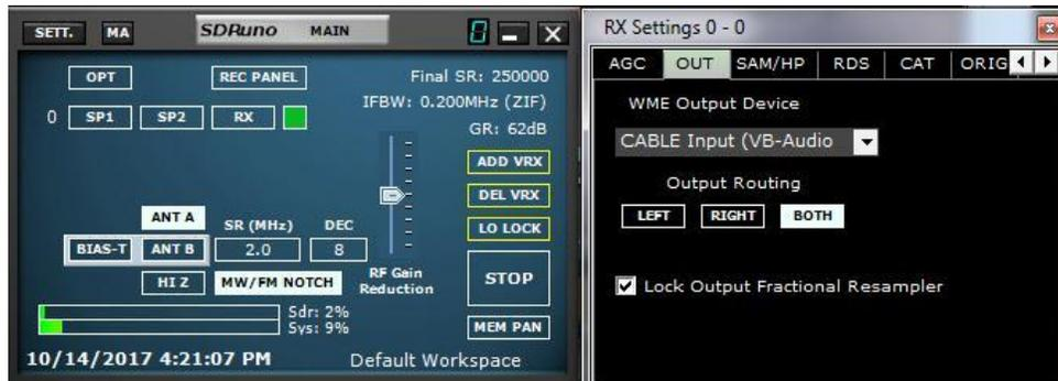
In MARS-ALE and MS-DMT you need to select your VAC output, in my case the VB-“Audio Cable Output” as the PCSDM input. You could also make the VAC the system default sound device as we are only talking RX with the RSP2pro receiver. There are some advantages in do this as some software used for audio recording just do not support other than the default sound device.
