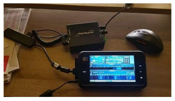
The use of the RSP2pro and its ability to record real-time RF spectrum to IQ .wav files have been invaluable in MS-DMT development efforts when channel conditions challenged the ability of MS-DMT modem performance.
