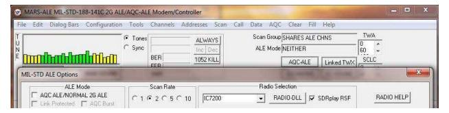
To keep the SDRplay RSP T/R support as simple as possible, the SDRplay RSP required VSP COM ports are specified as COM 20 for use in SDRuno and COM 255 in MARS-ALE. As such a Virtual Serial Port (VSP) Null Modem pair of COM 20 and COM 255 must exist.
