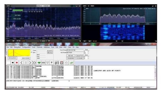
The RSP2pro and its SDRuno software can be used for intercept of multiple 2G ALE networks at the same time by configuring multiple virtual receivers (VRX) and VSP pairs for CAT control, enough VAC channels for RX audio with multiple instances of MARS-ALE.
