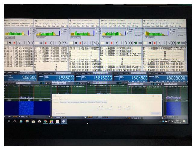
When used as a standalone receiver only, the low cost RSP2pro (\$192USD) can be used 24/7 unattended for 2G ALE ALL CALL based follow on data modem broadcasts with the more expensive transceiver physically taken out of the loop so as to protect it from lightening related damage.
